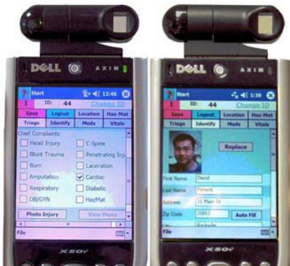
Fig. 3 PDA shows screens for inputting chief complaint (left) and for capturing patient photo (right)
