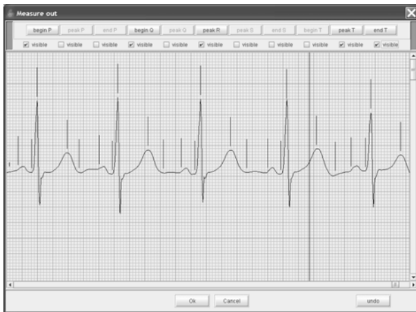
Fig. 11. Detail analysis display for P and Q wave onsets, R peaks and T waves peaks and offsets.
