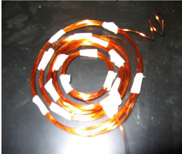
Figure 2: An experimental approximate figure showing a coil with only five bundles.
