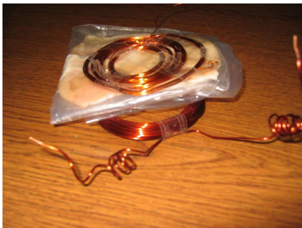
Figure 3: The primary (single-bundle) coil at the bottom separated by a 4 mm-thick fat layer from the secondary (multi-bundle) coil on top.
