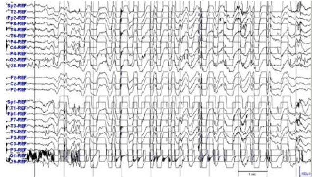
Fig. 2. False detection from patient 2 caused by reference electrode failure. Solid vertical line indicates the start of the 4 sec interval which caused the false detection. Light vertical lines indicate 1 s intervals.
