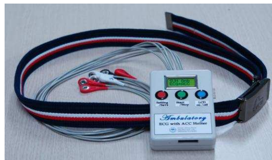
Figure 1. Instrument for data acquisition – 3 Ch ECG and 3 Axes' Accelerations
