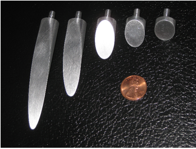
Fig. 4. Scaled needles of \text{Ø}1.5 cm used to understand the interaction between the needle tip and medium. Needles of various bevel angles ( 10^\circ , 15^\circ , 30^\circ , 45^\circ , and 60^\circ ) were used in the study.
