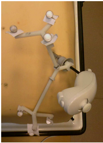
Fig. 8. Instrument with Nunchuck interface
