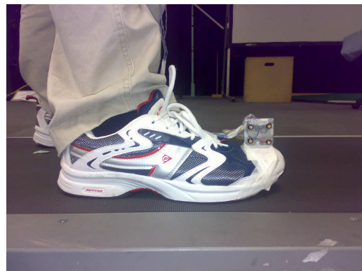
Figure 1: Experimental setup for monitoring toe displacement data with the Optotrak system.
