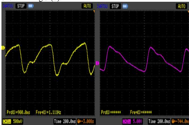
(a) Infrared pulse (b) Red pulse Fig.1 Example of red pulse and infrared pulse
