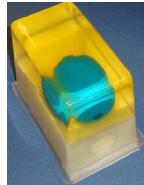
Figure 3. An ultrasound visible phantom was used to evaluate our compounding technique.
