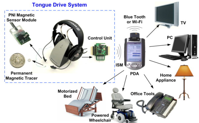
Fig. 1. Block diagram of the external Tongue Drive System (eTDS) prototype, built on a wireless headphone.
