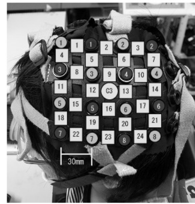
○ Illuminator ● Detector □ Channel
