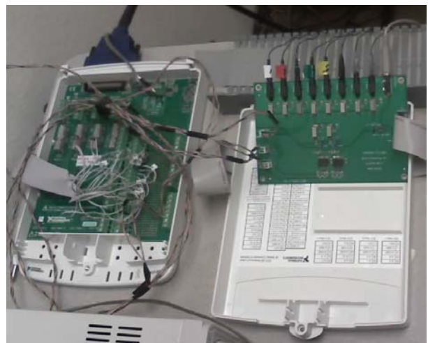
Fig. 5. Octopus system. On the left is the National Instrument SCC-68 I/O screw terminal board with its cable interface (black cable on top of figure) to the PCI card inside a desktop computer. On the right is the custom designed Octopus board diagrammed in Fig. 4, on top of the cover for the white SCC box. The 8 leads leading to skin electrodes, and the ground connector on the right, are shown on top of the Octopus board.
