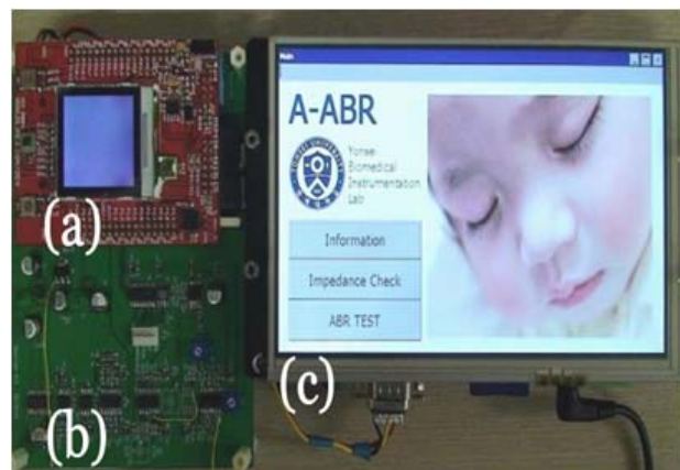
Fig. 1. Photo of a hardware; (a) Microprocessor, (b) Amplifier, (c) LCD
