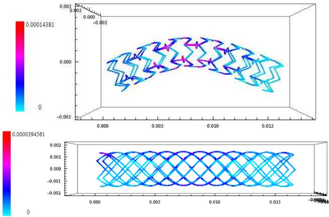
Fig. 2. The figure shows numerical simulation of a non-fractured Xience-like stent (top) and Palmaz-like stent (bottom) exposed to the same bending forces. Stent struts are colored based on the magnitude of contact moment. Much higher bending rigidity can be observed in the Palmaz-like stent (bottom).
