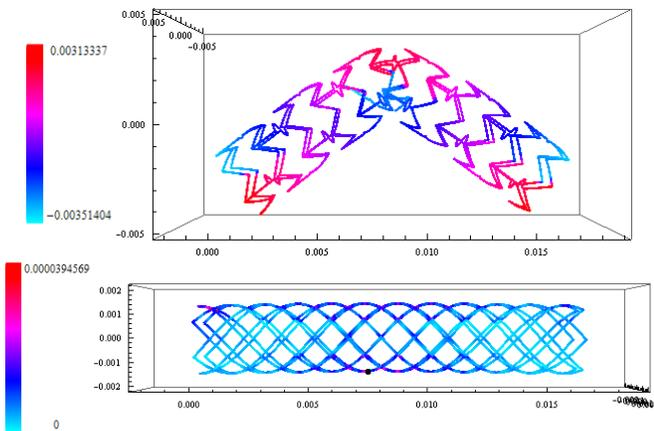
Fig. 3. The figure shows numerical simulation of a fractured Xience-like stent (top) and Palmaz-like stent (bottom) exposed to the same bending forces. The disconnected vertex lies at the bottom center of each stent (denoted by the black dot in the Palmaz-like stent at the bottom panel).
