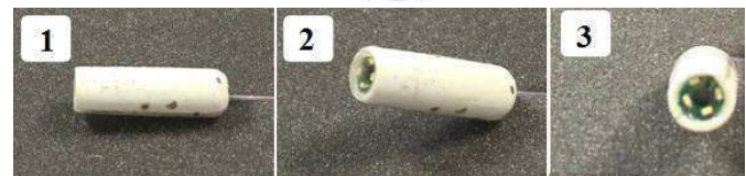
Fig. 8. MIM test on free space: three consecutive steps. The MIM and the external magnet are positioned respectively upon and under the surface of a table.
