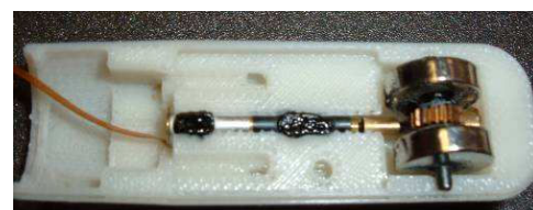
Fig.5. Half capsule body shell with the MIM.
