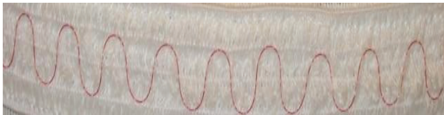
Fig.2 : Optical fiber embedded into textile during its process of fabrication
