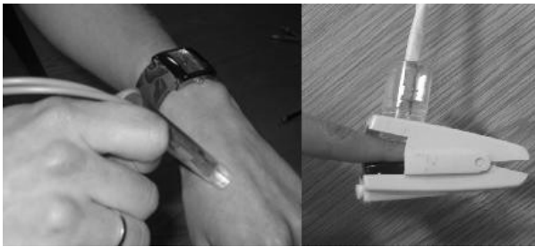
Fig.1. (a) Outline of Perspex rod and (b) the developed splanchnic fiber optic sensor
