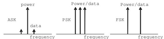
Fig. 2. Power spectrum of different modulation scheme.
