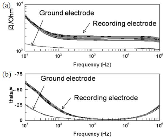
Figure 2. (a) absolute impedance,  $|Z|$  in Ohm and (b) the phase shift,  $\theta$  in degree plotted with respect to the measurement frequency
