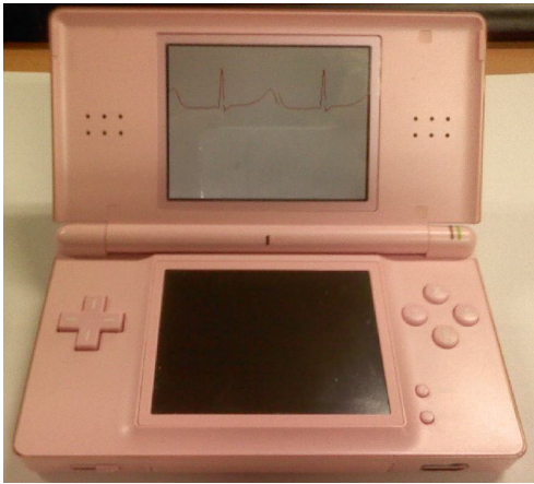
Figure 12 Bio-signal displays on to Nintendo DS LCD
