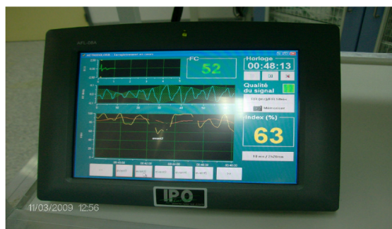
Fig 9. Real time monitor (Tablet PC) with ECG real time acquisition, RR series computation and filtering, and EnvTOTnu measurement.
