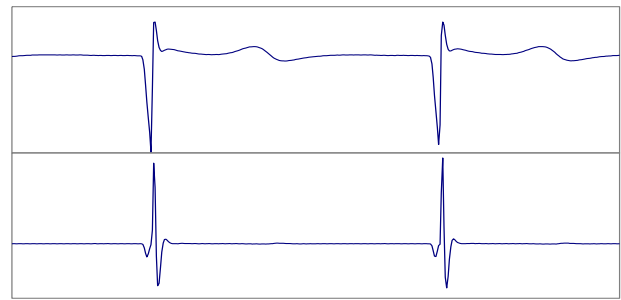
Fig. 10. Comparison of raw electrogram (upper) and filtered electrogram (lower) from ventricle.
