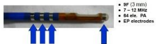
Fig 1. HockeyStick catheter with extra electrodes to enable electrofield 3D localization and image overlay. The catheter is 9Fr.
