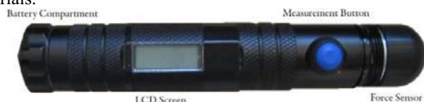
Figure 3 A prototype of a noninvasive central venous pressure monitor developed as a team's Honors project is portrayed
