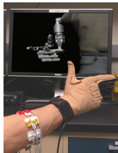
Fig. 1. A subject demonstrates control of the virtual prosthesis through use of the CyberGlove while EMG signals are simultaneously recorded.
