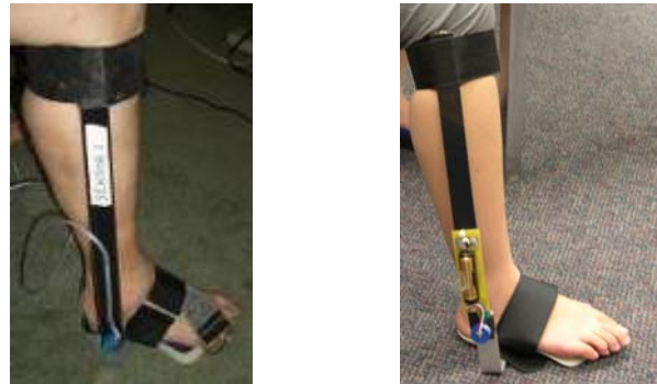
Fig. 8. Wired (left) and wireless (right) versions of the ankle sensor.
