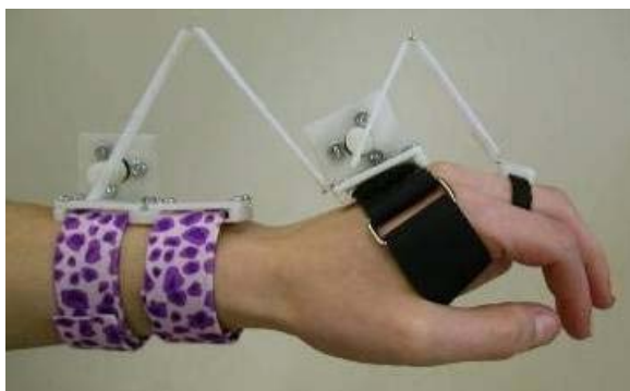
Fig. 3. Electrogoniometer with finger and wrist sensing.
