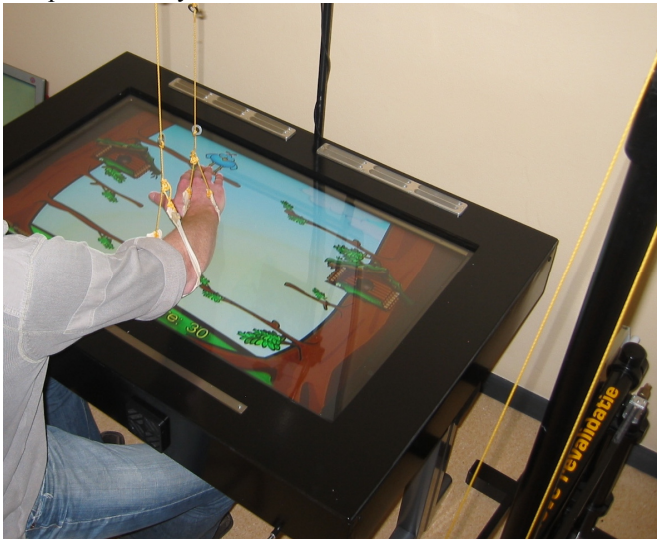
Figure 1. Gravity compensation device 'Freebal' (on the right) in combination with rehabilitation game 'FurballHunt' (table display)
