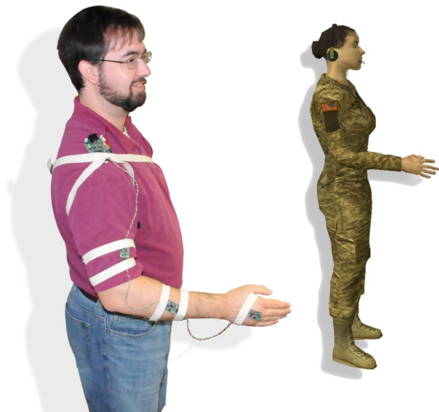
Fig. 7. Prototype system mounted on the right arm (left) and avatar controlled by the system (right).
