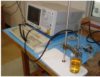
Fig. 1. Agilent 85070E dielectric measurement probe.
