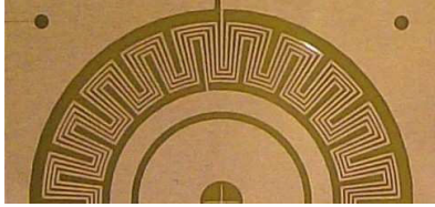
Fig. 6. Photo of a 200 \mu m linewidth planar coil etched on a copper-clad polyimide film (25 \mu m thick polyimide, 18 \mu m thick copper, 25 mm diameter, 4 mm radial linewidth length).
