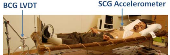
Fig. 4. The experimental setup. The subject lies supinely on the suspended ULF-BCG bed. An LVDT is used to measure the bed's displacement. An accelerometer is used to measure the SCG.
