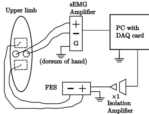
Fig. 1. Hardware setup of real-time tremor compensation.
