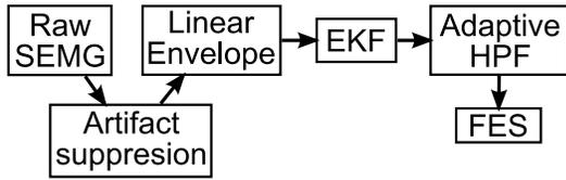
Fig. 3. Flowchart of the intended motion filtering algorithm
