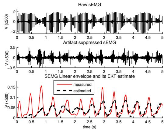
Fig. 6. Raw sEMG with FES artifacts(top); its linear envelope and the EKF estimate (bottom).
