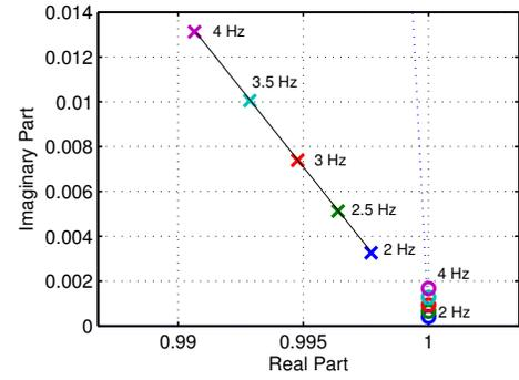
Fig. 4. Zero-pole plot of the high pass filters derived with brute force method. There are actually two roots but each is complex conjugate of the other.
