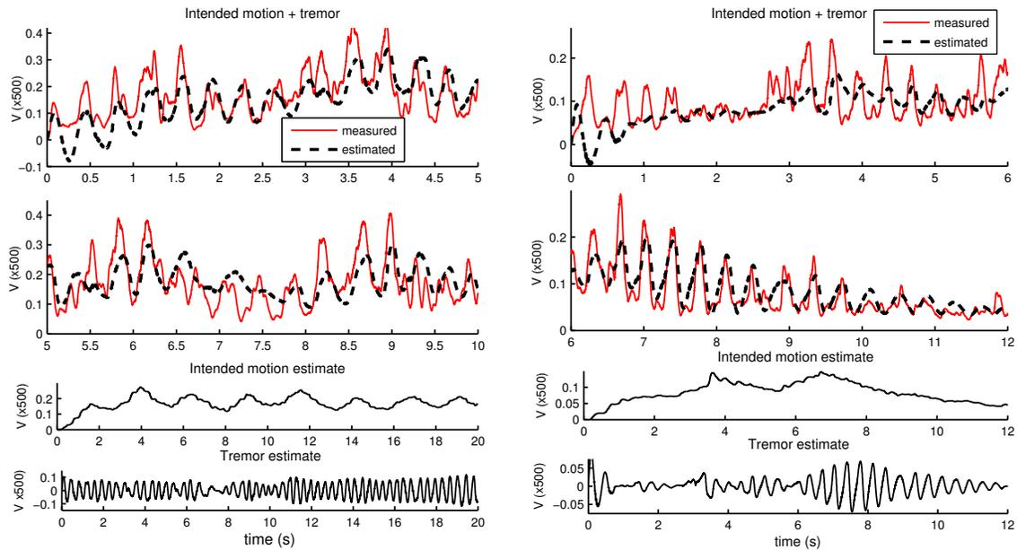
Fig. 5. Result of EKF algorithm to separate tremor from intended motion in finger to nose experiment (left) and Archimedean spiral drawing (right).
