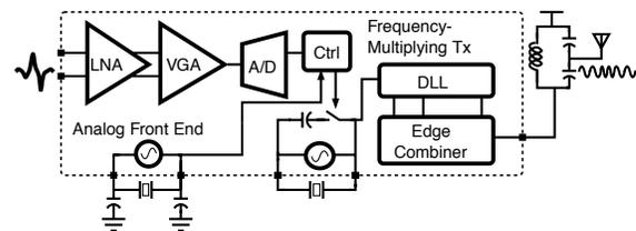
Fig. 3. Architecture of the wireless neural recording system.
