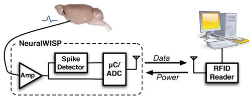
Fig. 6. System diagram of a wirelessly-powered neural sensor.
