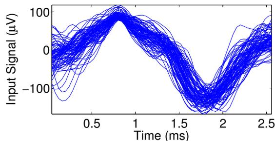
Fig. 5. Neural signals recorded *in vivo* from the motor areas of a rat brain using the analog front end described in III-B
