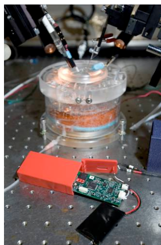
Figure 3. Photograph showing s WINCS unit and rechargeable battery in front, and background shows transparent interface style slice chamber with stimulating and recording electrodes.
