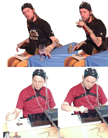
Fig. 2. Patient A with BCI and neuroprosthesis based on surface electrodes on the left hand (upper row) and patient B with implanted neuroprosthesis in the right hand.
