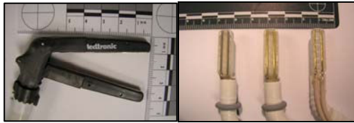
Fig. 2: Bipolar clamp device (left) and linear surface probe devices (right) with gold plated stainless steel electrodes.
