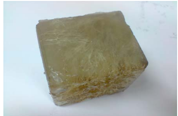
Fig. 3. The breast mimicking phantom was consisted of a solid epoxy base, clay spheres mimicking tumors, and agar branches mimicking breast tissues as mammary glands.
