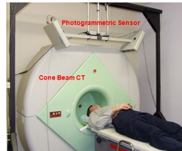
Figure 1: Fusion of CBCT and photogrammetric sensor
