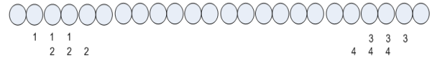
Figure 3: Four possible matching positions in the target image when the source bitewing image contains three complete teeth.
