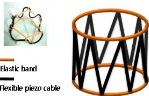
Fig. 2. The shape of the pMAS. The pMAS consists of an elastic band at each side and a flexible piezo cable between the elastic components
