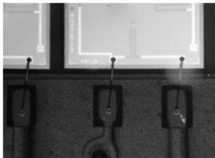
Fig. 4. Electrical connection between silicon chip and lead frame
