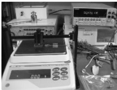
Fig. 9. Measurement setup for sensor output vs. hold down pressure
