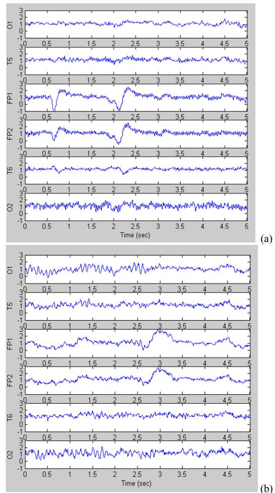
Fig. 5. EEG signals acquired using the proposed electrode system. (a) alertness EEG, (b) drowsiness EEG.
