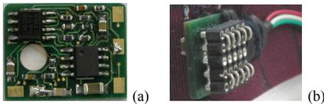
Fig. 3. Active dry electrode. (a) component side, (b) skin side. Skin side consists of 10 Ag-AgCl arc conduction points.
