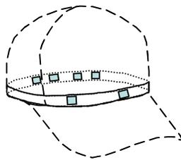
Fig. 4. Six active electrodes were arranged around a strip of Velcro, simulating the cap-ring, in the approximate location of Fp1, Fp2, T5, T6, O1 and O2.
