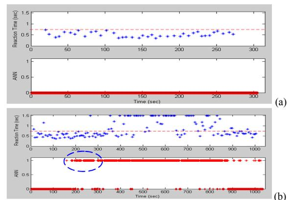
Fig. 7. Typical results of reaction time test (upper panel) and ANN detection results (lower panel) during (a) alert and (b) drowsy. Whenever the reaction time was longer than 700 ms, the subject was declared drowsy. The dotted circle indicates fault detection of drowsiness.
