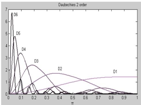
Fig. 2. The equivalent filters response of the stationary wavelet transform.
