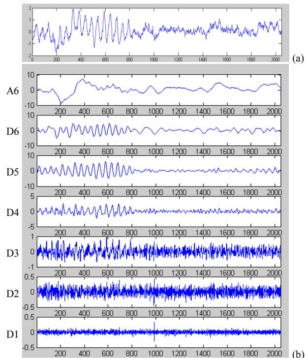
Fig. 6. (a) EEG signal and (b) the results of stationary waveform transform where D4, D5, and D6 contain the same frequency bandwidth as  $\beta$ ,  $\alpha$ ,  $\theta$ , respectively.
