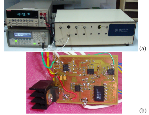
Figure 4: (a). Instrumentation set-up. (b). Analog PCB.
