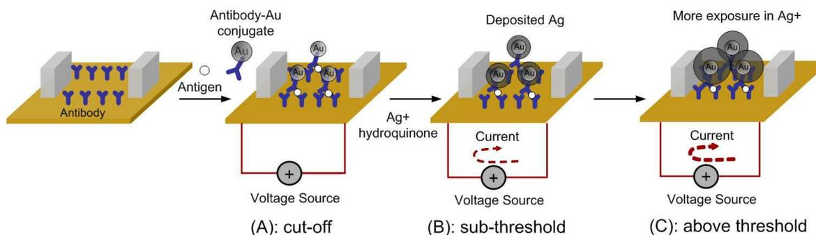
Fig. 1. The operating principle of the silver-enhanced biomolecular transistor with three distinct regions of the operation.
