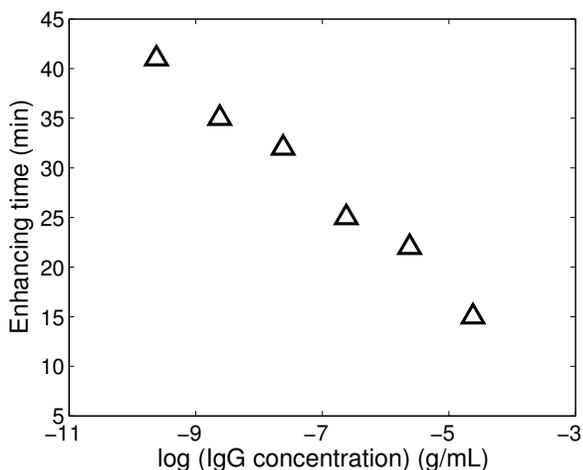
Fig. 6. Quantitative analysis: the silver enhancing time required to reach a conductance range of 3.8 – 5 mS as a function of gold particle concentrations.
