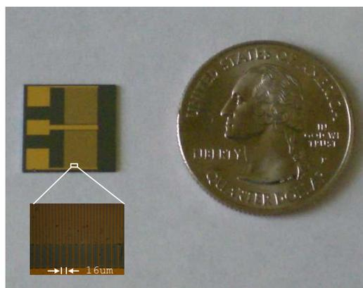
Fig. 2. The high-density interdigitated microelectrode biochip.
