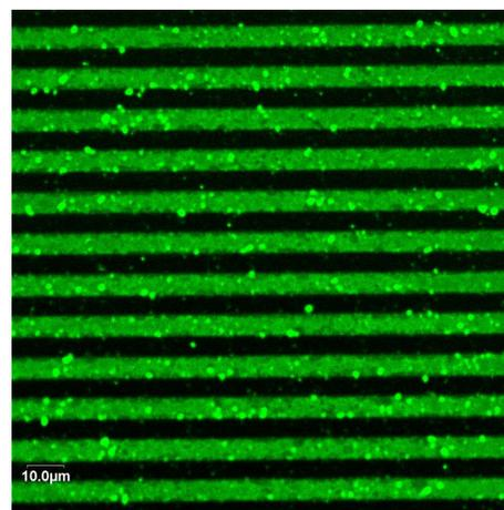
Fig. 3. Confocal laser scanning microscopy image of electrodes showing FITC-labeled bovine IgG only immobilized to silicon dioxide surfaces (black areas are the electrodes where no IgG are present).
