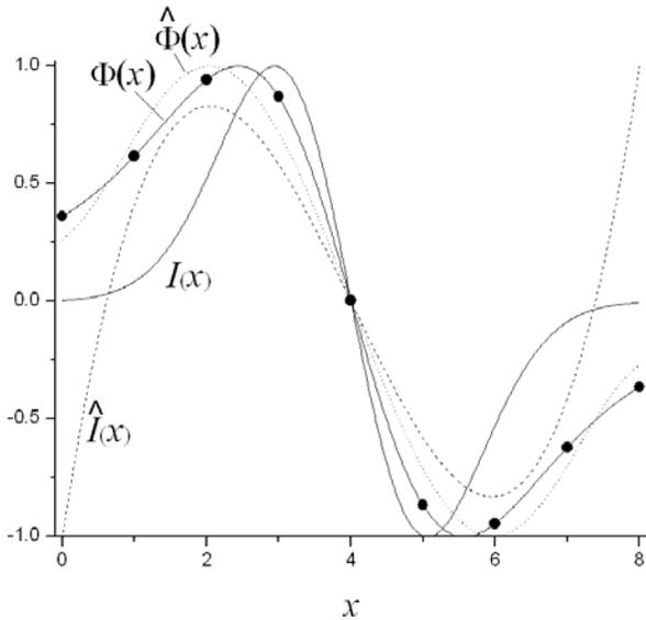
Fig. 2. The polynomial deconvolution method has difficulties with a more tortuous  $I(x)$  signal (compare to Fig. 1).
