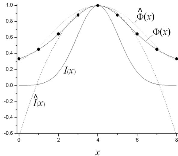
Fig. 1. A Gaussian  $I(x)$  is shown as the solid line. The potentials  $\Phi(x)$  that would be measured by 8 electrodes at a height of 1 above the tissue are shown as the filled circles. The estimate of  $I(x)$  provided by Eq. 4 is shown as the dotted line. The estimate of  $\Phi(x)$  provided by Eq. 5 is shown as the dashed line. All curves have been normalized to have a maximum of 1.0. Length  $(x)$  is in arbitrary units.
