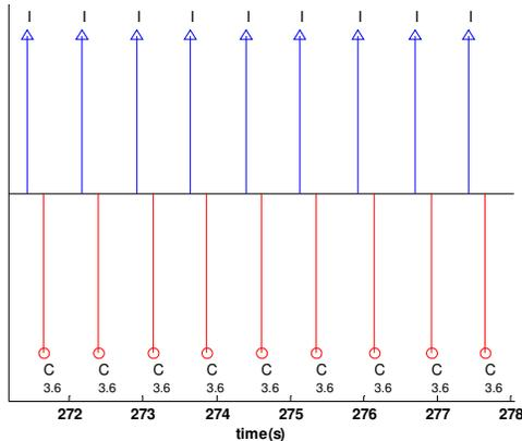
Fig. 2. A segment of simulated event markers for test case 8 while pacer operates in standard DDD mode. I – intrinsic AS, C – captured VP at 3.6V.
