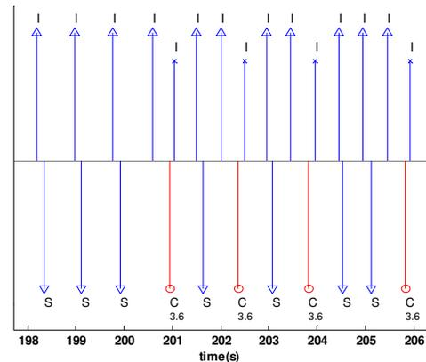
Fig. 5. A segment of simulated event markers for test case 15 while AVH is enabled. I – intrinsic AS ( $\Delta$  normal AS, x undetected AS in blanking window), C – captured VP at 3.6V, S – conducted VS.
