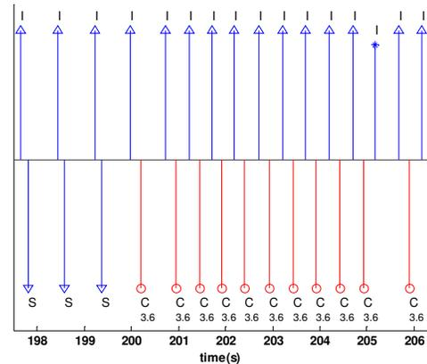
Fig. 4. A segment of simulated event markers for test case 15 while pacer operates in standard DDD mode. I – intrinsic AS ( $\Delta$  normal AS,  $*$  AS in refractory window), C – captured VP at 3.6V, S – conducted VS.
