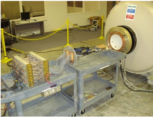
Fig. 5. 64 channel coil, tuning electronics, flange plate, T/R switch and preamplifier assembly prior to loading in the magnet.
