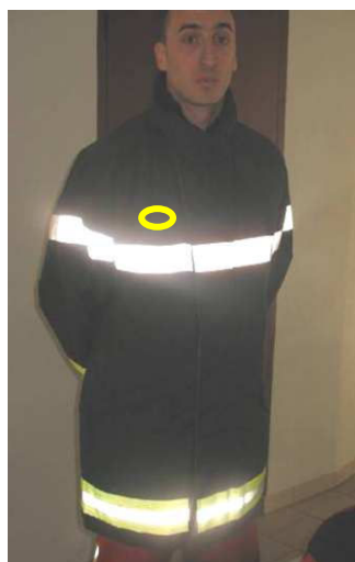
Figure 2: Sensors location in the outer garment (yellow circle). The temperature sensor is located under the external layer. The heat flux sensor is placed in a pocket under the internal layer.
