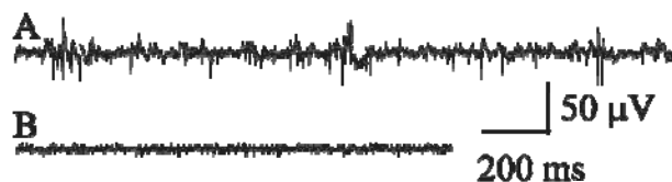
Fig. 1. A) Recording of spontaneous activity from a hippocampal slice culture placed on an SMEA after the latter was repeatedly stretched (one channel only). B) The biological origin of the signal was confirmed pharmacologically by eliminating spontaneous activity with 1μM tetrodotoxin.
